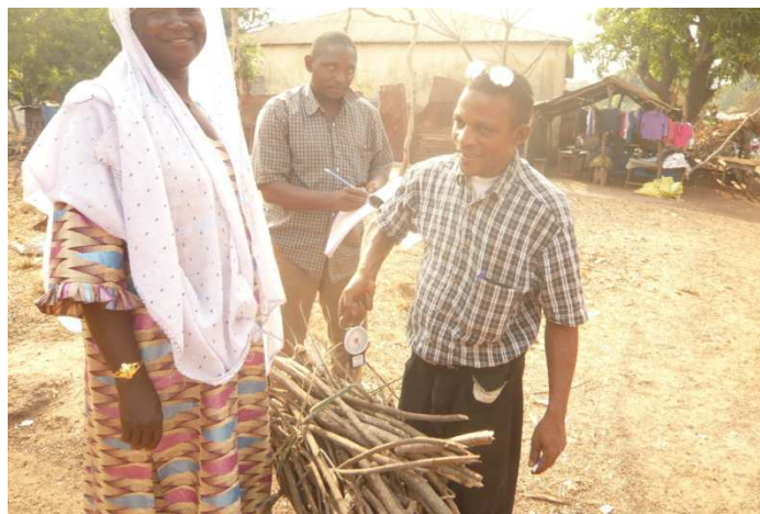
Wood fuel remaining stock weighting during the Kitchen Performance Test
